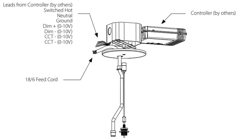
18/6 feed cord provided for wiring to pendant mounted SpectraSync luminaires. See table below for fixture to SJ cord connection recommendations.
